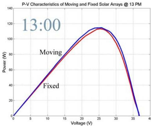
Fig.12: Power characteristics of movable and fixed PV-Arrays at 13:00
