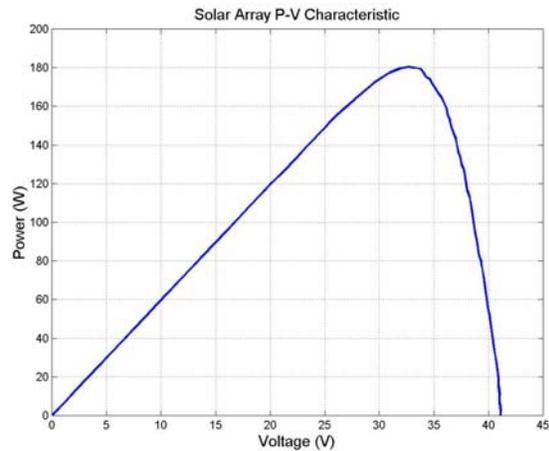
Fig.7: The output power curve of the PV-array at the standard condition
