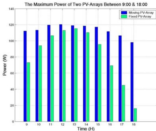
Fig.20: The maximum output power of two PV-arrays between 9:00 & 18:00
