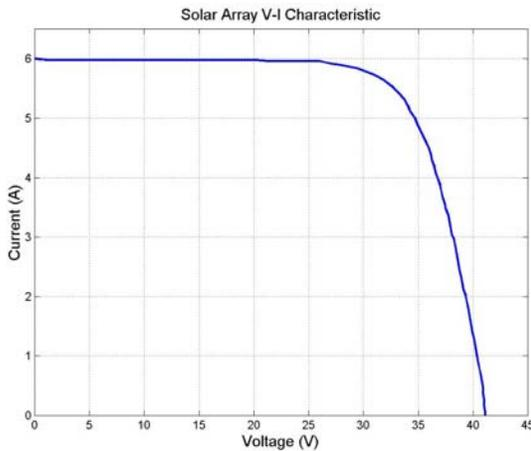
Fig.6: The output current curve of the PV-array at the standard condition
