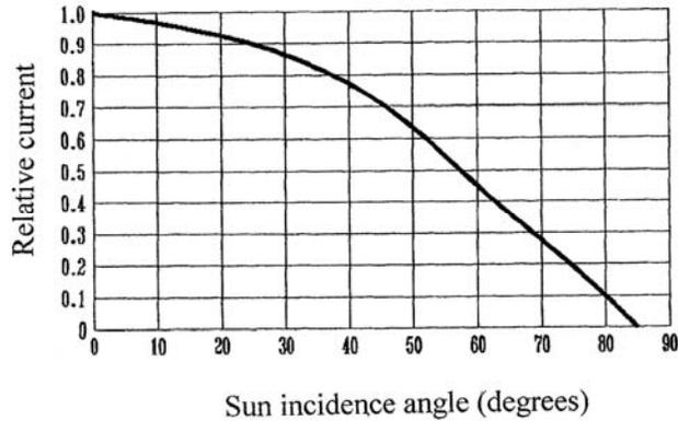
Fig.3: Solar cell current variation due to variation of the sun light radiation angel on the surface of the solar cell [2]
