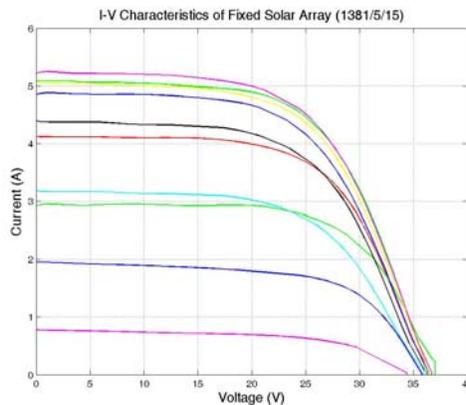
Fig.22: The output current curves of the fixed PV-array between 9:00 & 18:00
