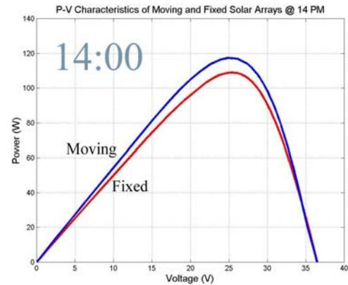
Fig.13: Power characteristics of movable and fixed PV-Arrays at 14:00
