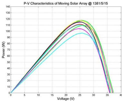
Fig.18: The output power curves of the movable PV-array between 9:00 & 18:00
