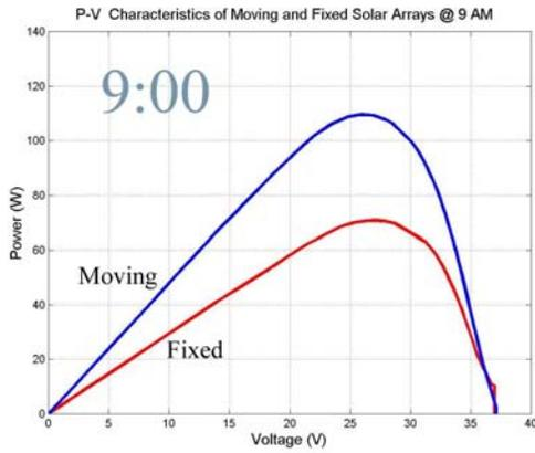
Fig.8: Power characteristics of movable and fixed PV-Arrays at 9:00
