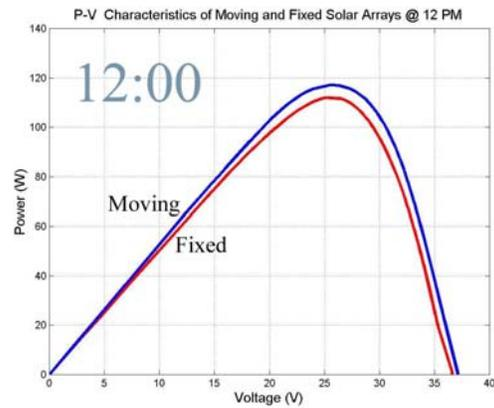
Fig.11: Power characteristics of movable and fixed PV-Arrays at 12:00
