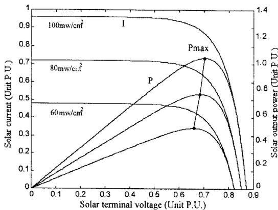
Fig.1: Variation of sample solar cell output characteristics with light intensity changes [3]
