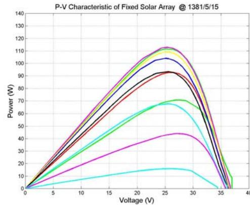
Fig.19: The output power curves of the fixed PV-array between 9:00 & 18:00
