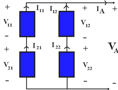
Fig.5: The photovoltaic array configuration mounted on the tracker
