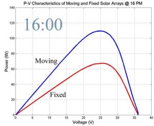
Fig.15: Power characteristics of movable and fixed PV-Arrays at 16:00
