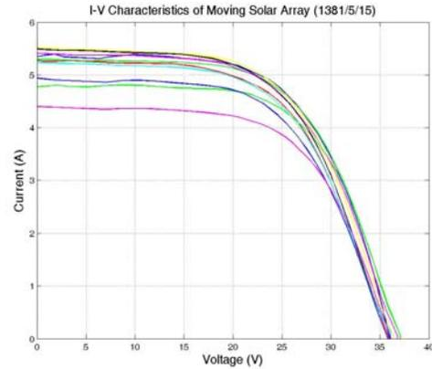
Fig.21: The output current curves of the movable PV-array between 9:00 & 18:00
