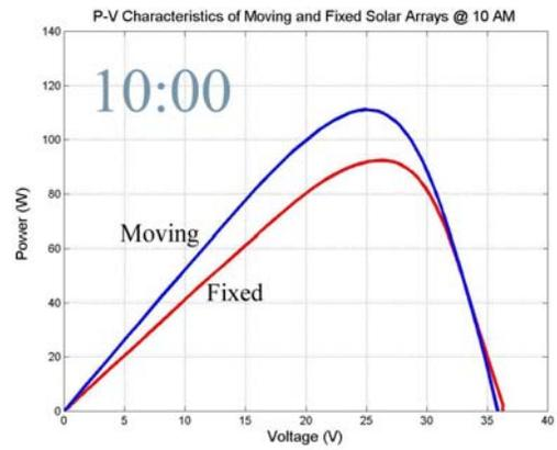
Fig.9: Power characteristics of movable and fixed PV-Arrays at 10:00
