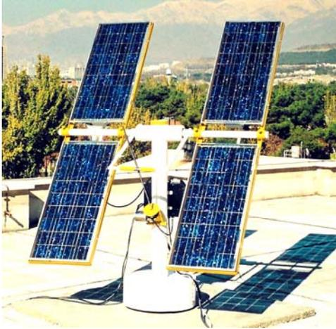
Fig.4: The two-axis Photovoltaic tracker implemented for the survey
