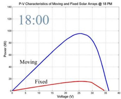
Fig.17: Power characteristics of movable and fixed PV-Arrays at 18:00
