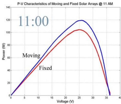
Fig.10: Power characteristics of movable and fixed PV-Arrays at 11:00
