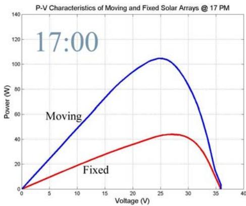
Fig.16: Power characteristics of movable and fixed PV-Arrays at 17:00
