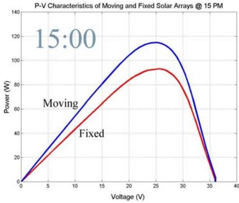
Fig.14: Power characteristics of movable and fixed PV-Arrays at 15:00
